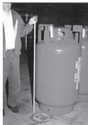
Photo 19 - Cylinder of halon 1211 (bromochloro difluoromethane).
