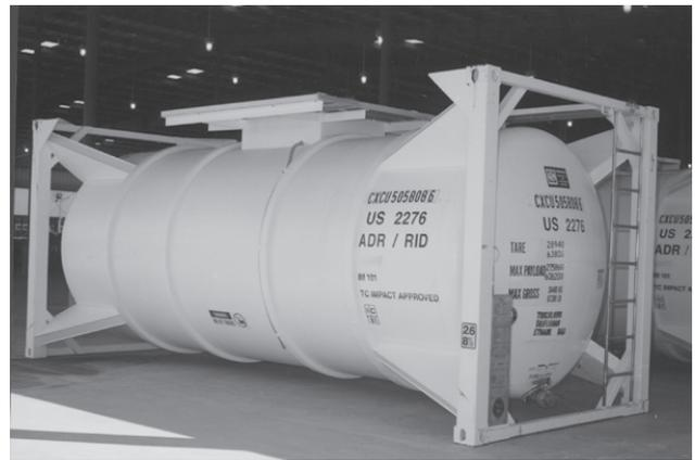
Photo 16 - ISO tanks allow for multimodal transport of large quantities of refrigerants.
