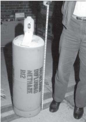
Photo 9 - Example of CFC-12 cylinder, dichlorodifluoromethane.
