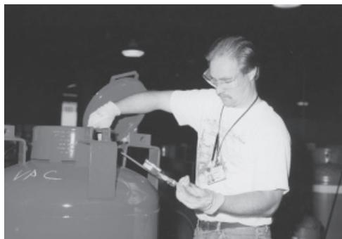
Photo 2. Conducting a temperature-pressure test.
