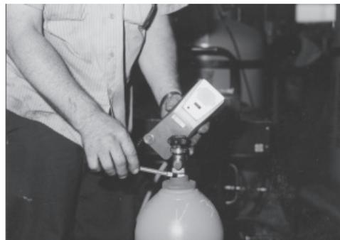
Photo 3. Example of leak detector.
