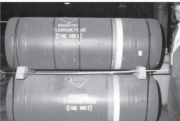
Photo 18 - Barrel of halon 1301 (bromotrifluoromethane).
