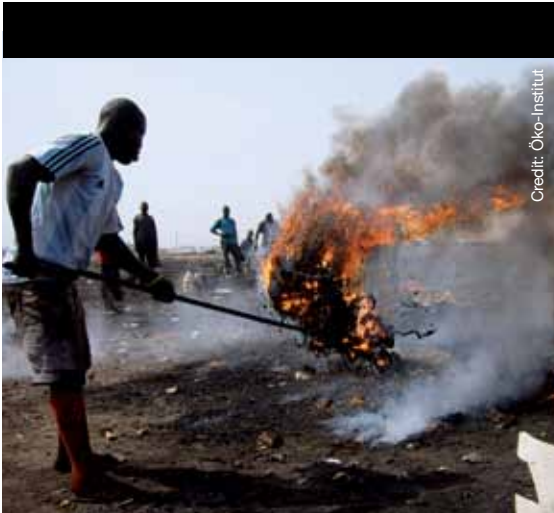
Burning cables, monitor and TV casings leads to severe emissions of harmful substances.
